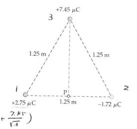
$$V = V_1 + V_2 + V_3 = \frac{2 \times 8.87 \times 10^3 \times 10^6}{1.25} \times \left(2.75 - 1.72 + \frac{7.45}{\sqrt{3}}\right)$$
